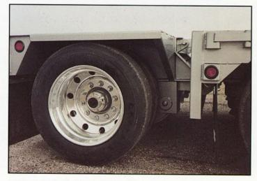
Optional covered flip axle is available for better utilization of rear deck space and increased scalability. Booster applications also available to assist in meeting multi-state maximum axle regulations.
