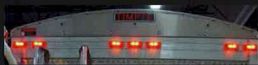
L.E.D. Seven (7) Lights on Rear Header Four (4) Outside Lights Turn/Clearance Three (3) Inside Lights Stop/Clearance
