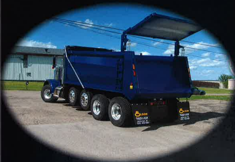
IN-POST AIR HIGH LIFT TAILGATE
