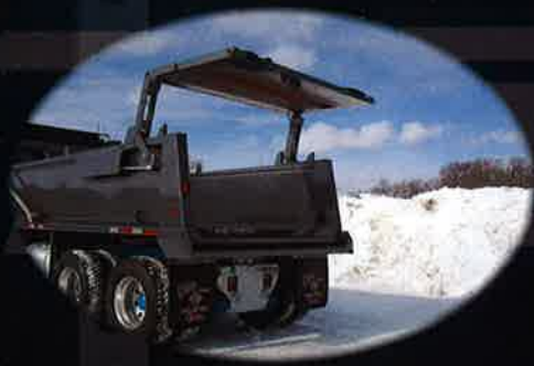
OUTSIDE MOUNT AIR HIGH LIFT TAILGATE
